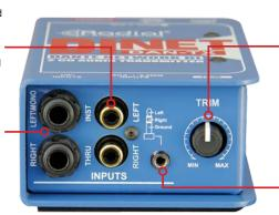
TRIM - Adjustable Trim control to set input levels, with unity gain at 12 o'clock. Provides -10dB of cut or +10dB of gain at the min/max settings.
